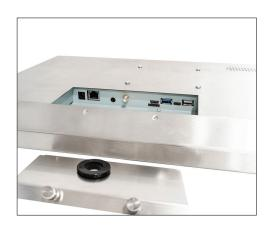
Power over ethernet (POE) eliminates the need and expense of electrical outlets at each station, as well as, power supplies and cable management requirements that typically accompany other KDS hardware solutions. This will reduce points of failure, which then makes it easy to trouble shoot and provides the ability to easily support & service.
