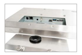
Power over ethernet (POE) eliminates the need and expense of electrical outlets at each station, as well as, power supplies and cable management requirements that typically accompany other KDS hardware solutions. This will reduce points of failure, which then makes it easy to trouble shoot and provides the ability to easily support & service.
